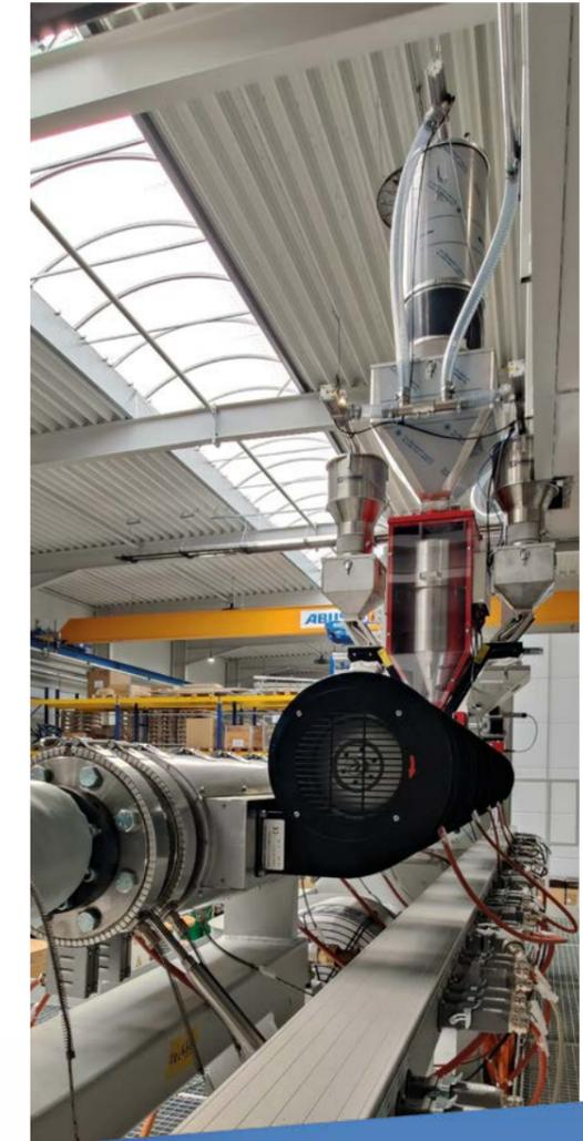
While the third pipe is under production, the first pipe is dismantled from the mandrel. The mandrel is going back to the first winding station for the next production sequence.
