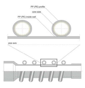
The core tube has to provide a high ring stiffness under extreme heat (up to 230° C) and at the same time it has to be flexible enough to be wound around the smallest pipe diameter produced with bauku machines, which is the DN 300. As the stiffness of the profiles produced with the inner core tube has to be different depending on the pipe diameter and the stiffness class, we at bauku have designed four core tube sizes to optimise our production.
